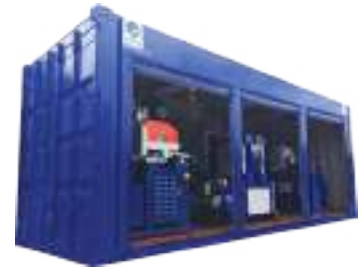
Bartec rebar preparation equipment installed in container
