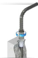
Position Type C is similar to Type B, with the addition of a lock-nut to maintain the second bar in position.
