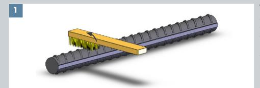
The reinforcing bar shall be free of any excessive dirt, concrete slurry, rust, etc. that may affect product performance.
