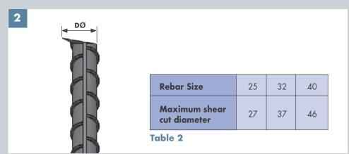
Maximum shear cut diameter shall not exceed the limit in table 2.
