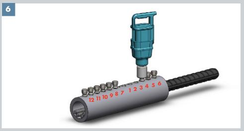
Tighten the bolts, from centre to outside (1 to 12), with a hand wrench or power drive (pneumatic wrench) until the heads of the screws shear off.
