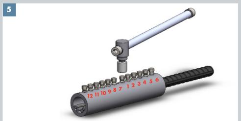
Hand tighten the bolts from centre to outside (1 to 12) with a wrench to pre-position the coupler.
