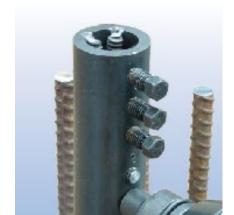
Tighten the screws, from centre to outside, with an impact wrench until their heads shear off. manual wrench can be sufficient for small quantities).
