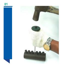
Remove the center pin with a punch.
