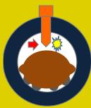
The bar is oval, and the bolts are in front of its smallest side, so their tips don't touch the bar.
