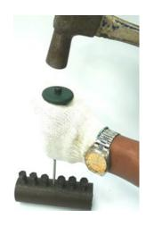
Remove the center pin with a punch.
