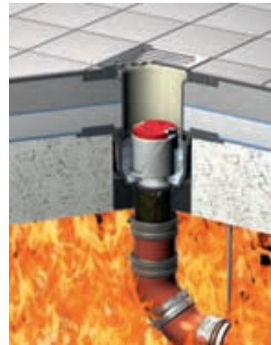
A fire on top of the ceiling expands. The intumescent mass in the odour seal to completely block the drain
