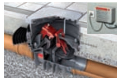
ACO Quatrix-K black water automatic backflow stop, DN 100 Type 3F pursuant to EN 13564 for installation in floor plates.
