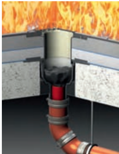
If a fire is present beneath the ceiling, the intumescent mass in the cartridge safely blocks the socket in the drain
