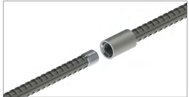
Figure 5: Straight metric threads. The ends of the rebar are cold forged to increase their diameter, prior to threading.
